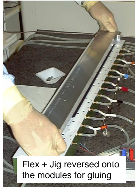
Flex before gluing and assembly onto Silicon modules
