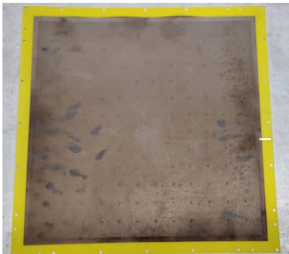
25 cm × 25 cm THGEM foil && Resistive PCB
