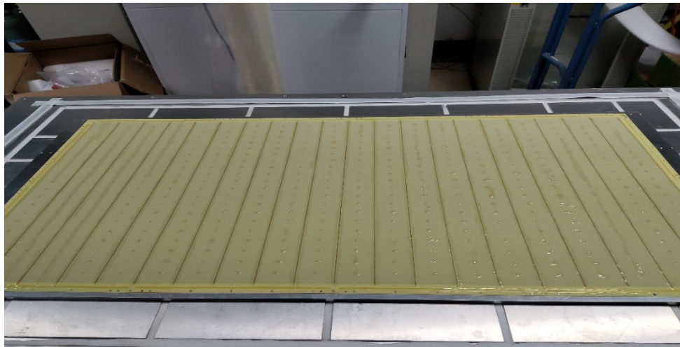
Gluing area of the THGEM PCB
