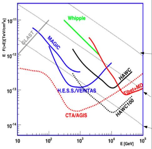
New generation of VHE gamma-ray telescopes will allow increase of sensitivity by a factor of ~10 compared to the present generation instruments.
