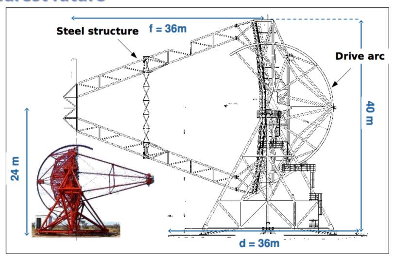
HESS collaboration is currently building a larger size telescope (dish diameter 27 m, collection area  $^{\sim}600 \text{ m}^2$ ) to achieve a lower energy threshold  $E_{\nu}>50 \text{ GeV}$ .
