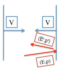
Energy gain for a particle reflected from a moving shock wave (Lorentz transformation)
