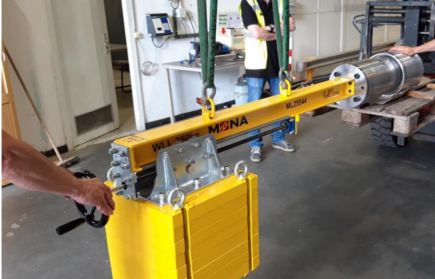
Collimator insert and lifting spreader test
