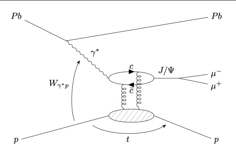
the J/ $\psi$  goes in the direction of the Pb ion: 702 GeV <  $W_{\gamma^*p}$  < 1486 GeV
