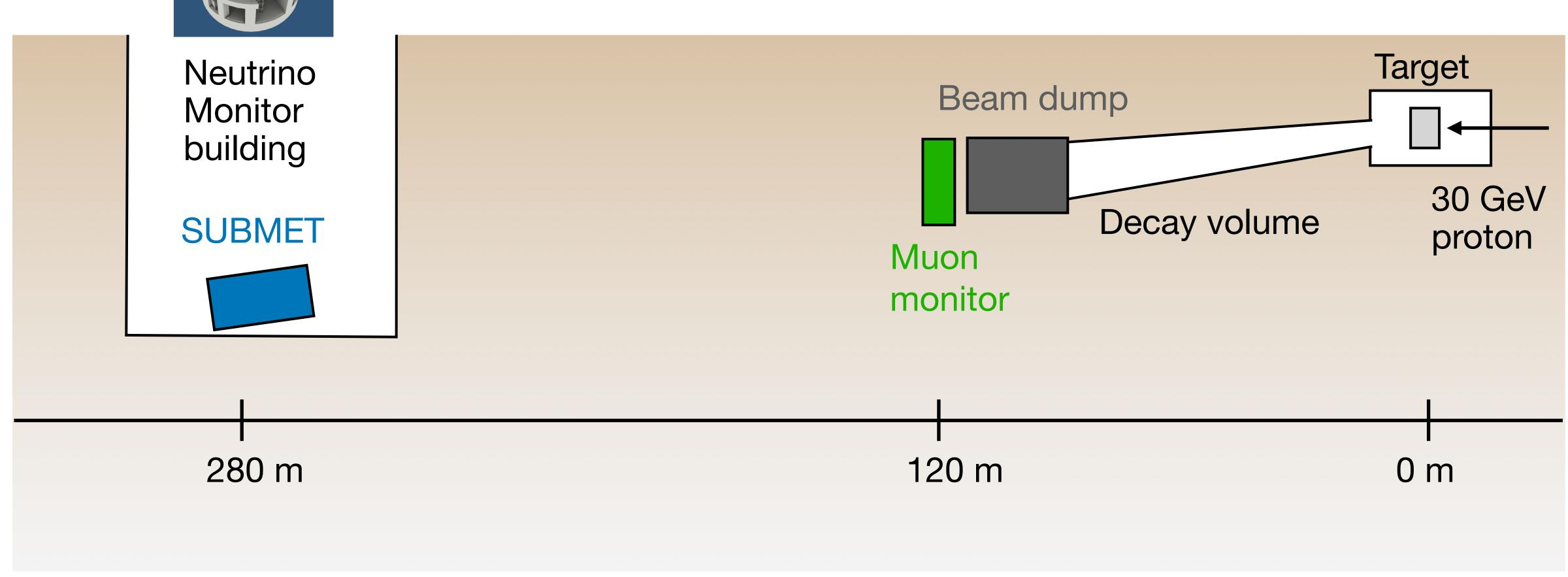
Protons hit the target and produce hadrons
