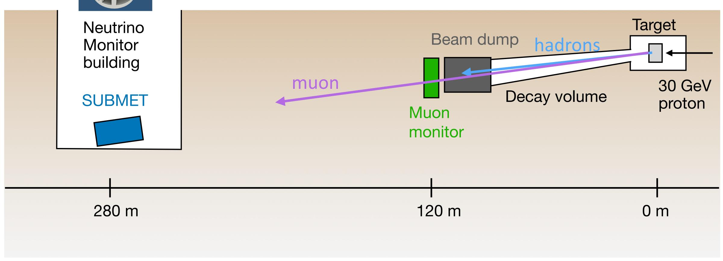
Muons pass the beam dump, but lose energy in sand (5 MeV/cm) before reaching the Neutrino Monitor building
