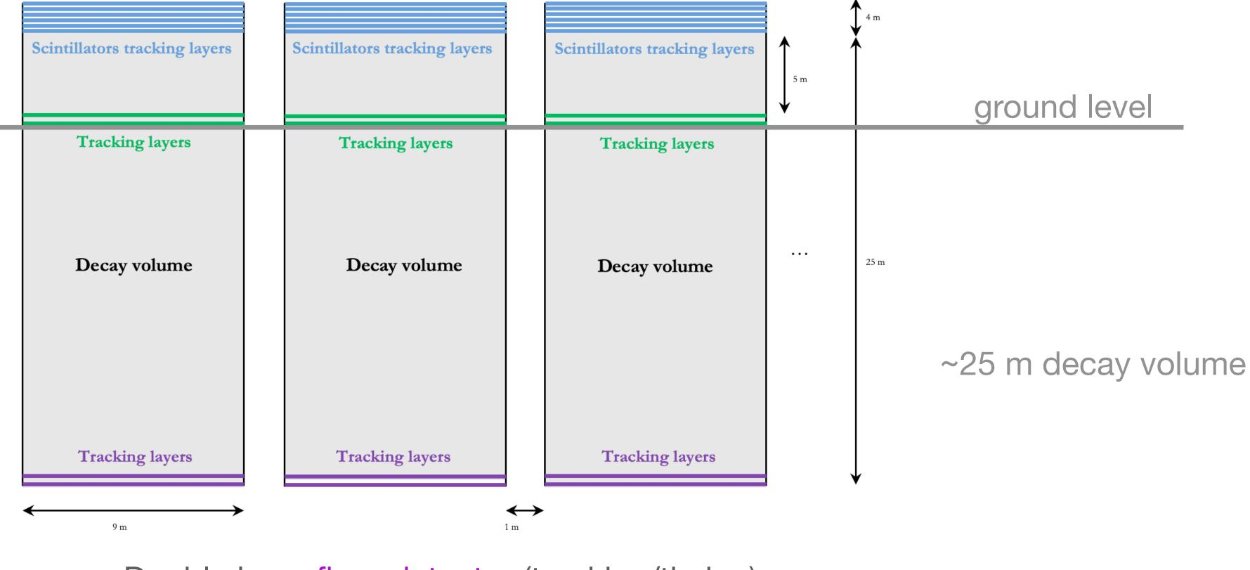
Double layer floor detector (tracking/timing)
