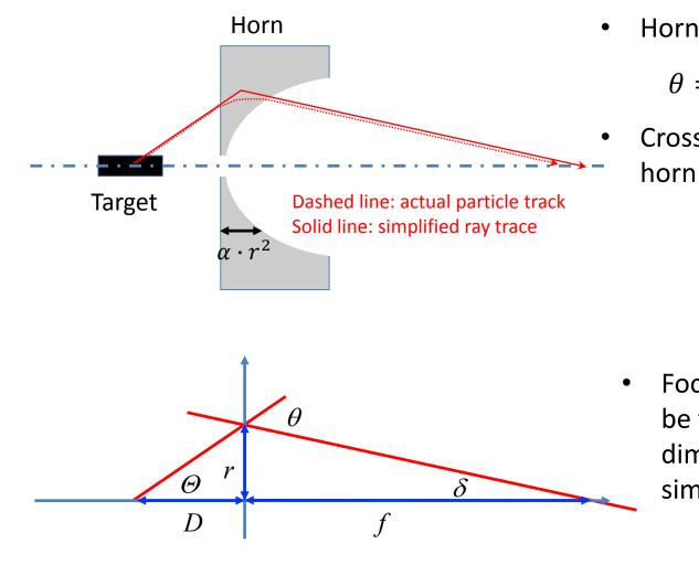
Horn focusing force  $\theta = \frac{eb_{\varphi}l}{\cdots} \propto \frac{I \cdot r}{\cdots}$  $p_z p_z$ Cross-sectional shape of
