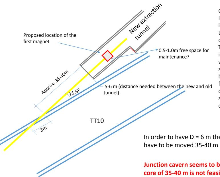
Courtesy of K. Balazs In order to allow the structural integrity of the existing and new tunnel we would need to keep a certain distance between the two. This distance it is marked with "D", in our case the TT10 being 4 m wide that would mean approximately 5-6m distance between the two tunnels in the first 10-15 m, but in order to confirm we need to do a proper alignment drawing to see the exact dimensions.
