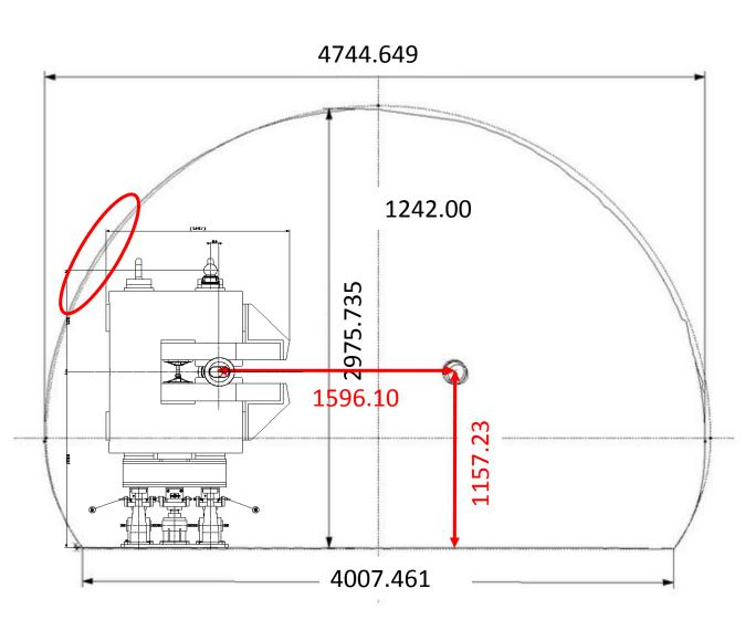
5 switch magnets each providing 0.0405 rad → 1037 mm offset (without drifts) → Total angle wrt walls = 11.6°
