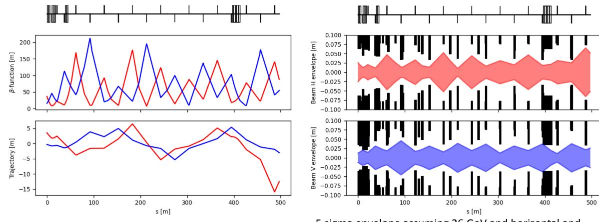
5 sigma envelope assuming 26 GeV and horizontal and vertical normalized 8 um and 6 um respectively
