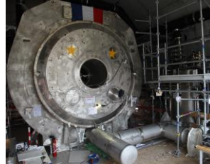
11,7T WB MRI magnets (NbTi conductor) (68 cm bore NIH-NRI magnets from ASG, 90 cm bore for Iseult CEA)
