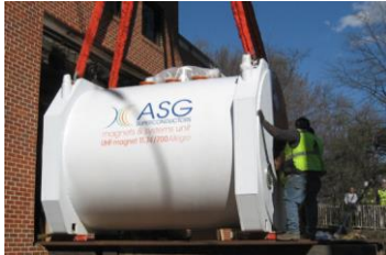
11,7T WB MRI magnets (NbTi conductor) (68 cm bore NIH-NRI magnets from ASG, 90 cm bore for Iseult CEA)
