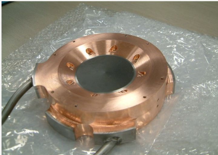
Fixed target, from 2008 to 2014 Lifetime: Irradiation damage of graphite 1 year at 1 MW operation
