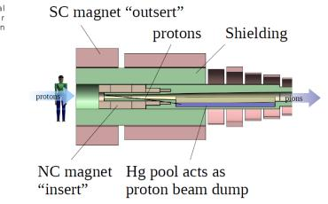
Hybrid design (superconducting + conventionnal magnets)
