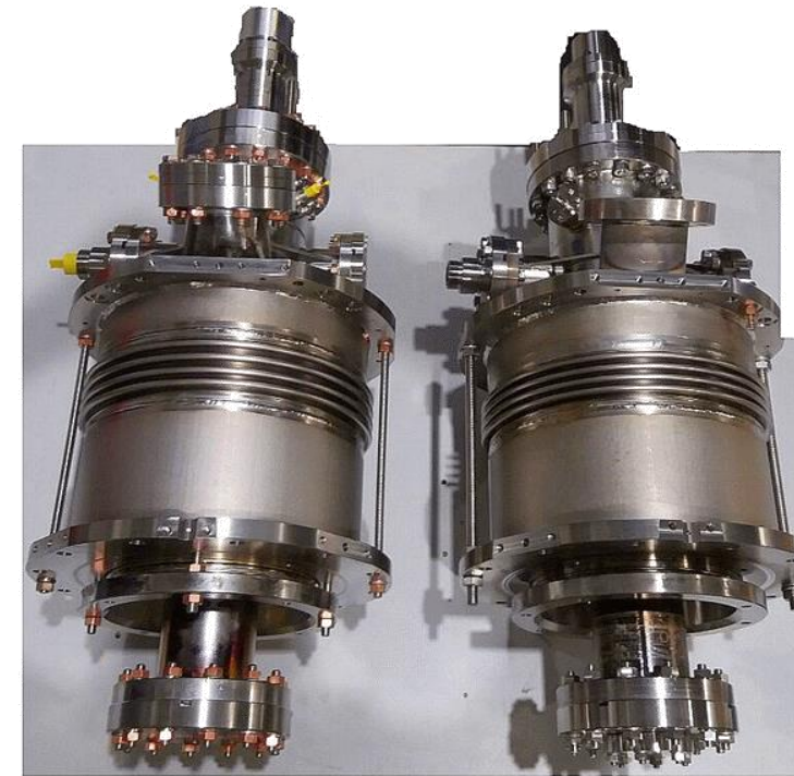
Cavities for operation with Cs 2 KsB photocathodes
