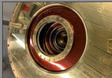
REX Linac 9Gap anodic capacitor repair (courtesy C. Gagliardi)
