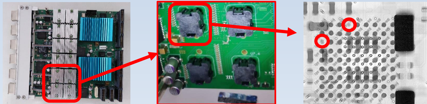
Missing balls from ball array
