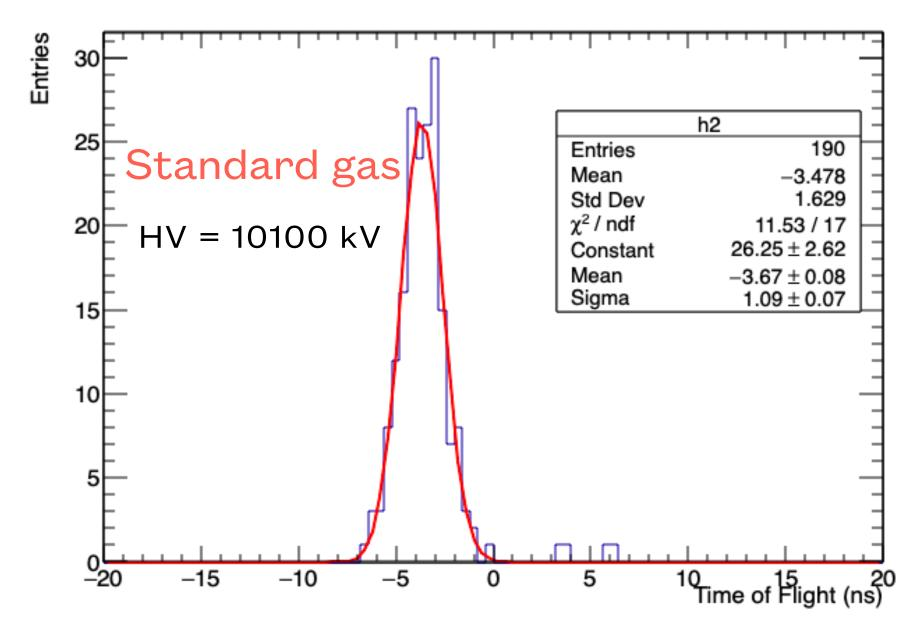
• Time resolution measured with the time of flight (TOF) method, using the 0.5 mm gas gap as time reference
