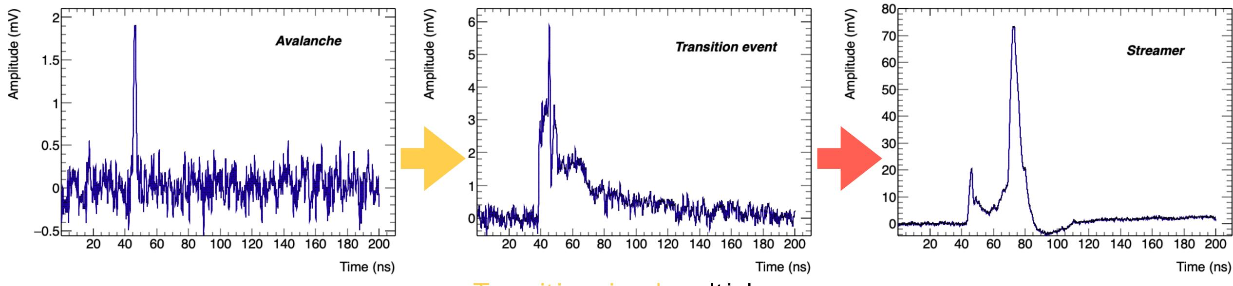
Avalanche: very short single signal  Transition signal: multiple avalanche signal and/or a large tail following the precursor
