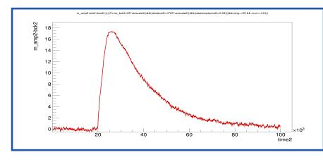
Ionic signal :read out on a resistance on the ground graphite electrode equal to 10 kOhm
