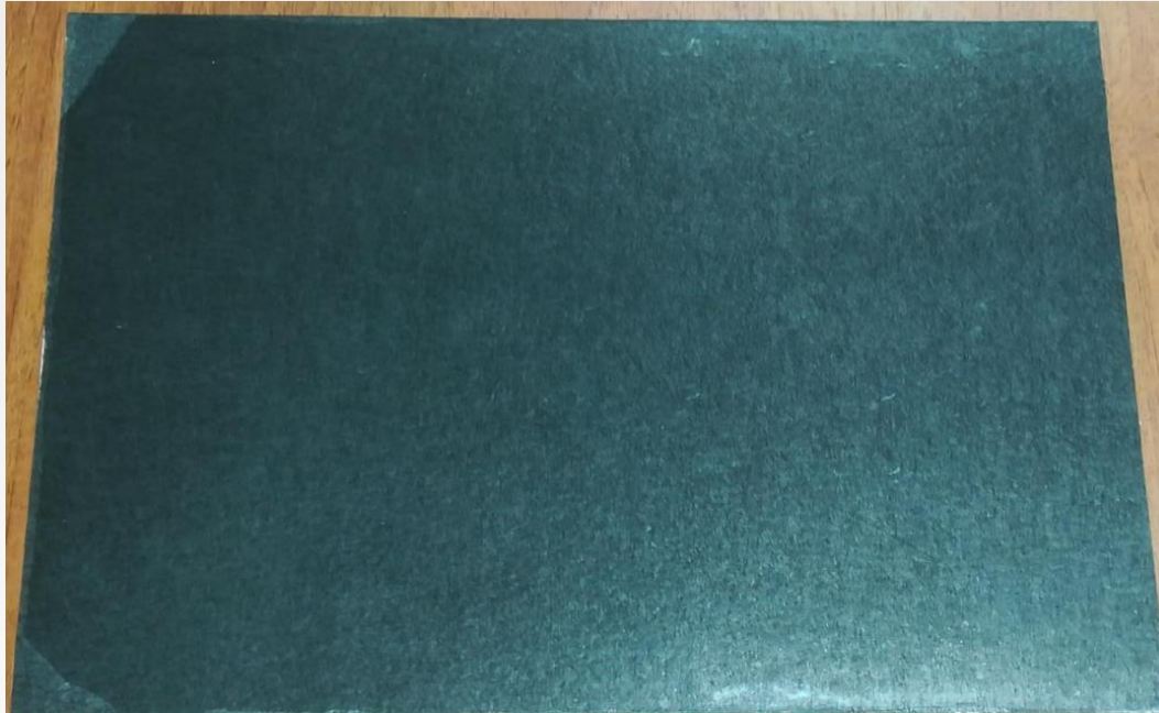
• Figure 12: Sandwiched Carbon Fiber sheet 200 mm x 290 mm x 0.3 mm
