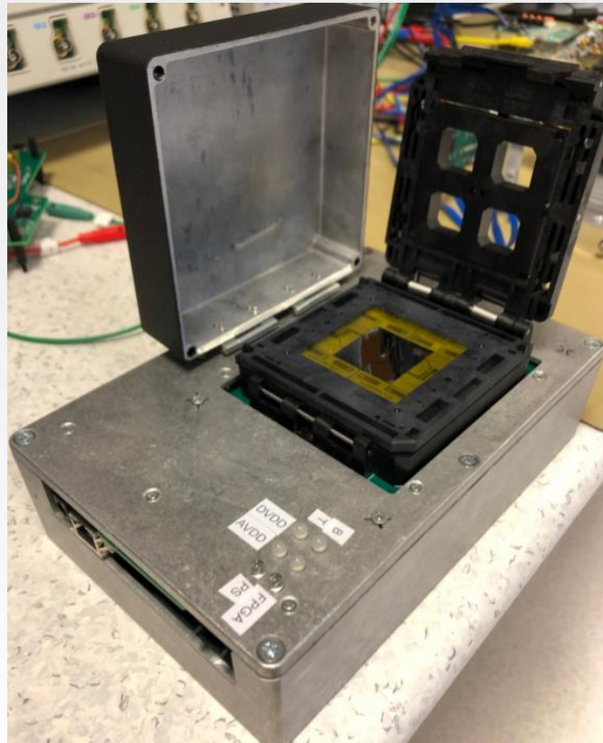
• Figure 10: Photograph of the production test box used for verification of the ALPIDE sensors after bonding.
