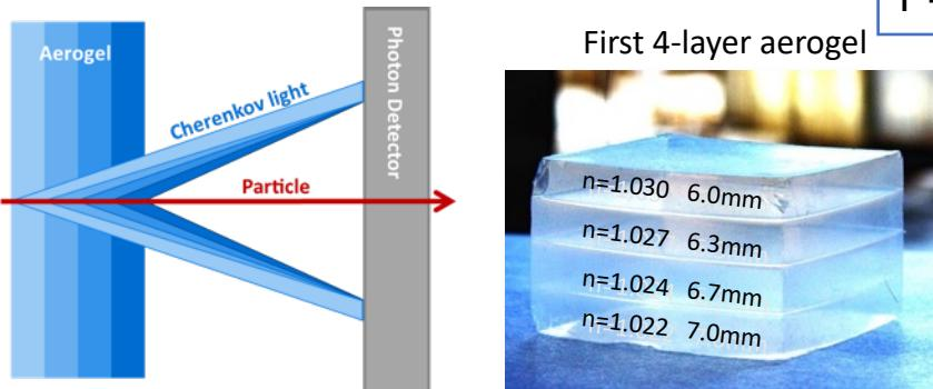
2012 test beam:  $\mu/\pi$  separation  $> 3\sigma$  at  $P=1$  GeV/c was demonstrated
