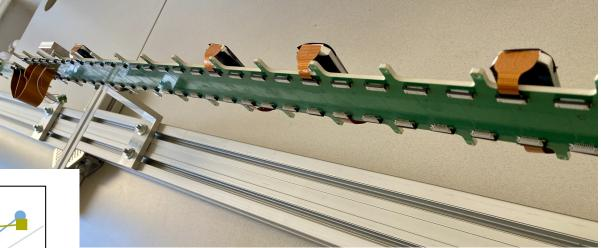
The longer the electrical connection line – the longer the time delay between detector hit and time stamp in the electronics.
