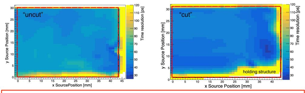
The overall average time resolution of both scintillators is much better than the design goal: **53.1 ± 4.3 ps** for "uncut" scintillator and **41.5 ± 5.1 ps** for "cut" scintillator.
