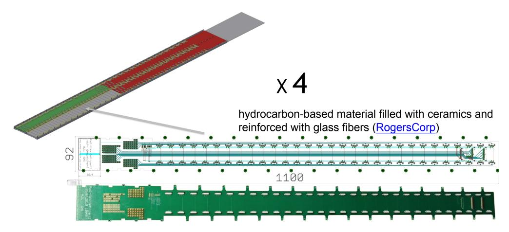
...connects the Front End Electronics (FEE) to the detector elements while providing mechanical support
