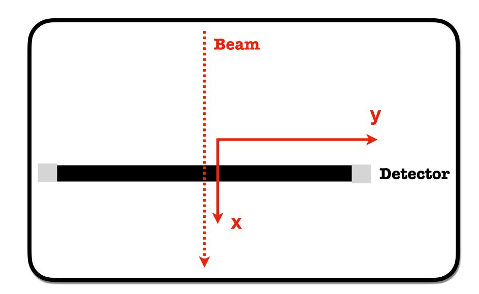
The beam entrance has been moved along the detector axis. The response is function of the solid angle, as expected.
