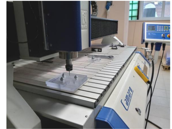
drilling three orthogonal through holes in each cube on the machine
