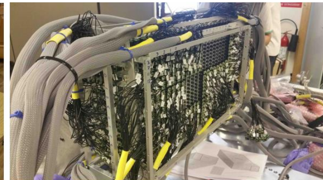
Left: the SuperFGD Prototype assembled with the fishing line method Right: the partially instrumented SuperFGD Prototype bottom face
