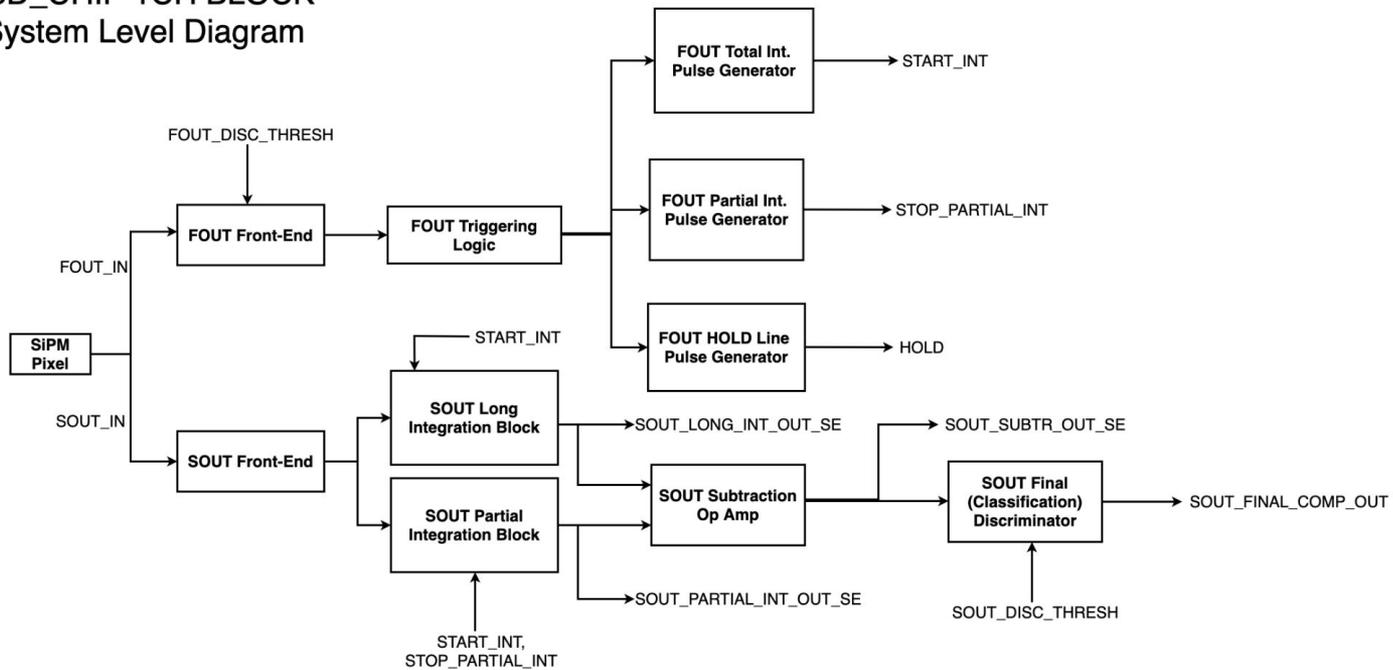
**SensL SiPMs provide a capacitively coupled fast output (FOUT) and a resistively coupled standard output (SOUT)**
