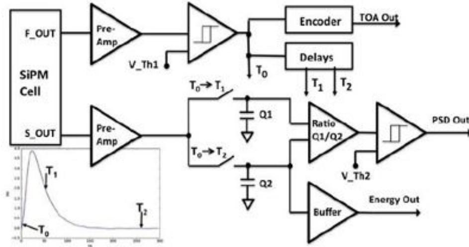
SensL SiPMs provide a capacitively coupled fast output (FOUT) and a resistively coupled standard output (SOUT)
