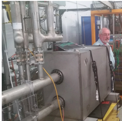
Test of fast-ramping normal-conducting magnet design
