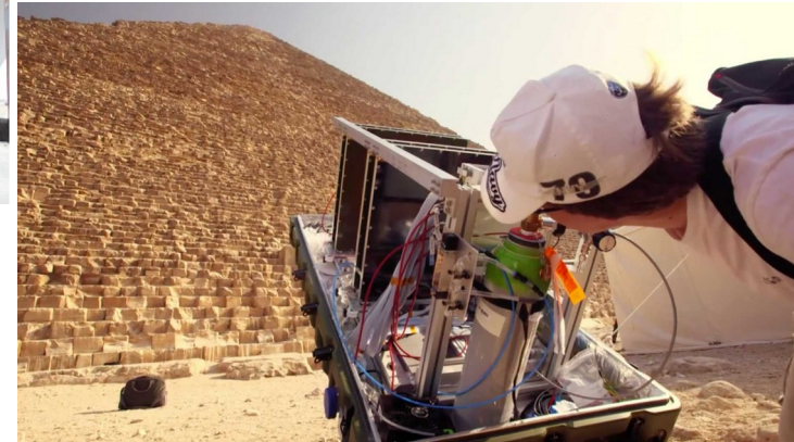
"Discovery of a big void in Khufu's Pyramid by observation of cosmic-ray muons", Kunihiro Morishima et al.
