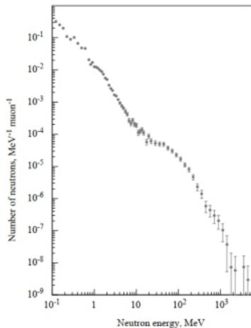
Cosmic muon-induced neutron spectrum
