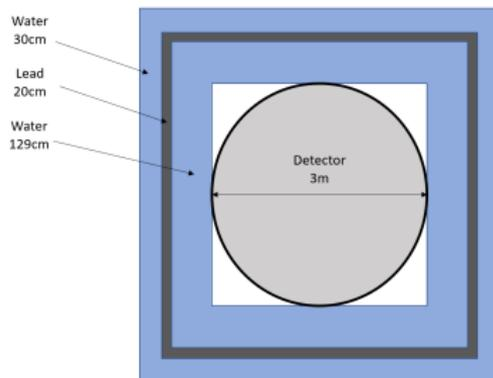
Diagram of a 7m cube water and lead shielding setup
