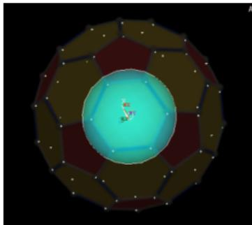
60-anode ACHINOS simulated with ANSYS - anodes are white points at the vertices of a truncated icosahedron
