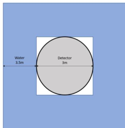
Diagram of a pure water shielding setup with 3.5m thick water on each side
