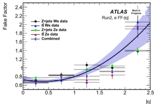
→ Combined points from weighted average of data FFs of Z+jets and  $t\bar{t}$ , weights are the respective statistical errors
