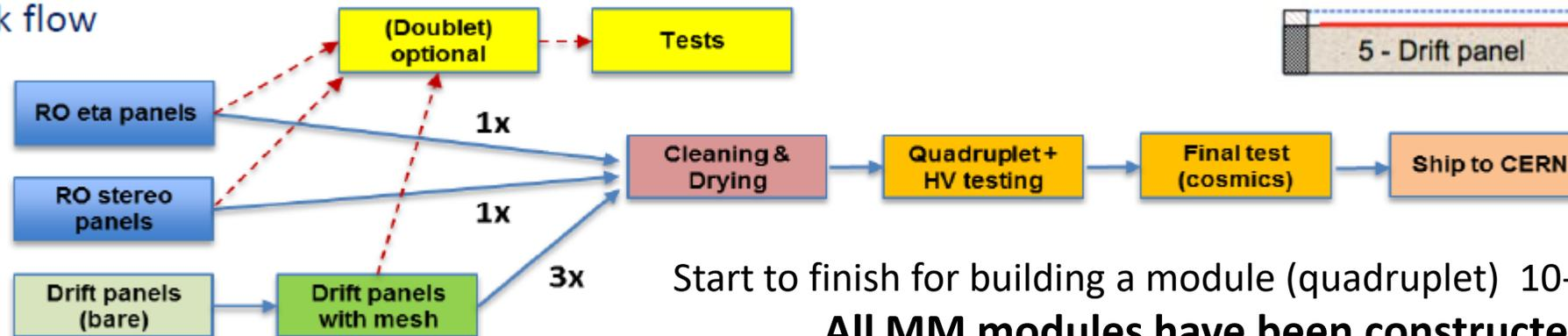
Start to finish for building a module (quadruplet) 10-12 weeks
