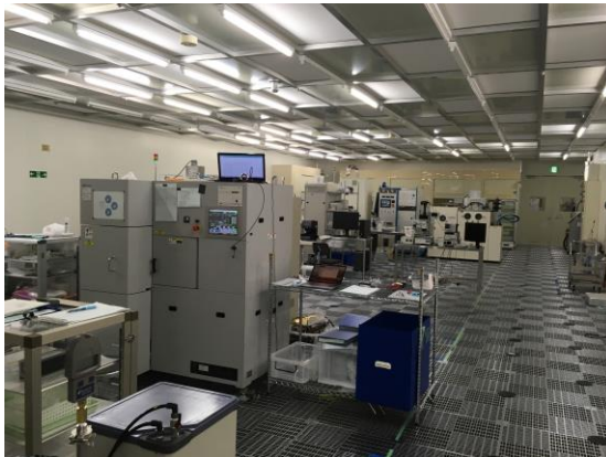
sputtering machine in the clean room (class 100)
