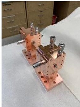
C-band Cavity (@LANL/@SLAC cold)
