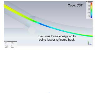
increase electron accelerating voltage to 15 kV
