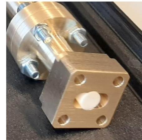
Alumina-loaded circular waveguide ø6 mm to WR 28 transition
