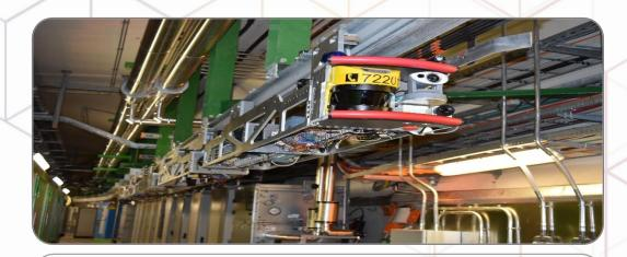
Train Inspection Monorail (TIM) is a unique modular, extensible, robotic platform capable to accomplish autonomously a variety of different missions. Including regular inspections, safety tasks, monitoring, complex interventions and others.
