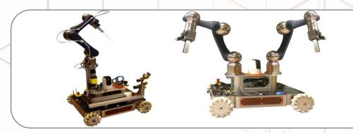
CERNBot is a modular and flexible robotic platform capable of delicate interventions in presence of ionization radiation. Primarily aimed for indoors interventions. Used across the CERN accelerator complex for critical interventions.
