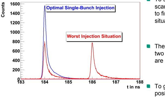
To set the gun delay, a scanning process was done to find the worst injection situation
