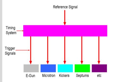
The distribution of the trigger signals are controlled by a timing system
