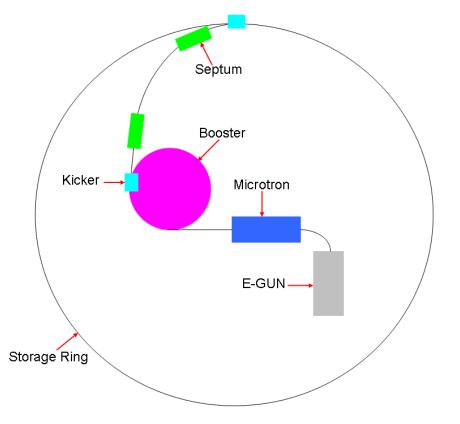
Electrons are generated from an E-Gun and pre-accelerated e.g. in a microtron and a booster
