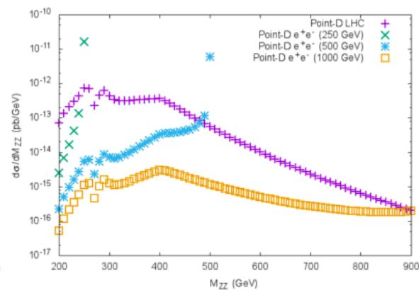
The differential  $\bar{f}f \rightarrow Z^* \rightarrow ZZ$  cross section at hadron and lepton colliders
