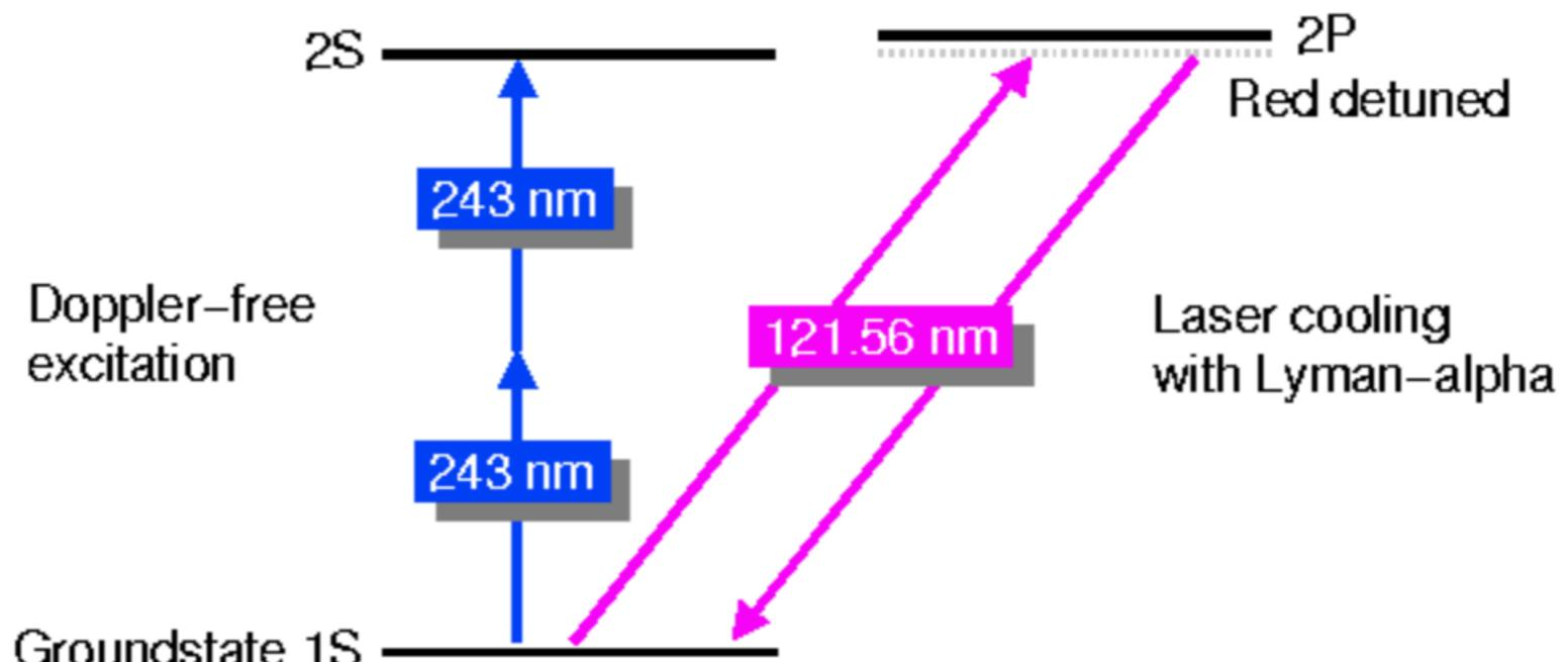
Simplified level scheme of (anti-)hydrogen showing only the lowest lying states and ignoring all substructure.
