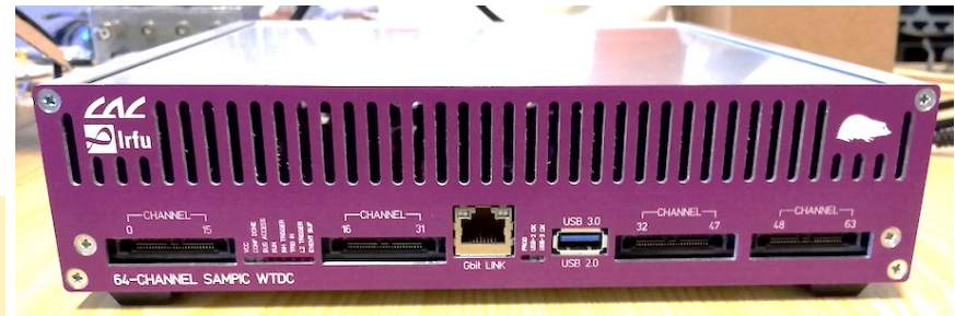
64-channel module with 16- channel input connectors (can be analog or differential digital)
