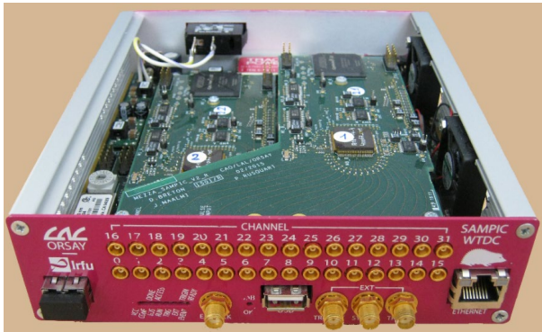
16 or 32-channel module (1 or 2 mezzanines)
