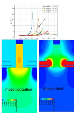
wider upper electrode shields field from the lower electrode
