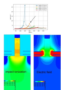
a wider lower electrode pushes field towards read-out electrode.
