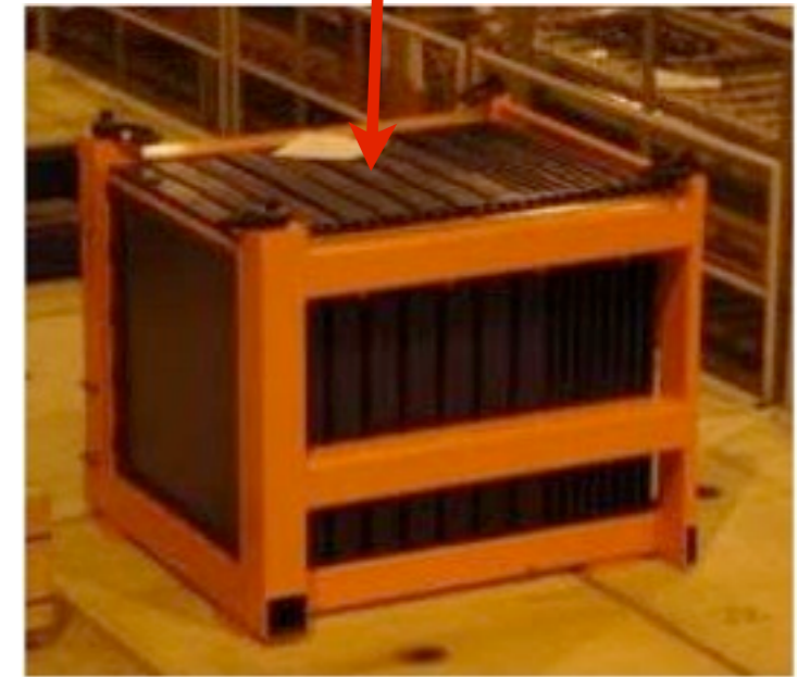
Tail Catcher / Muon Tracker 5 \times 100 \text{ cm}^2 Scintillator Strips 16 layers \sim 300 channels
