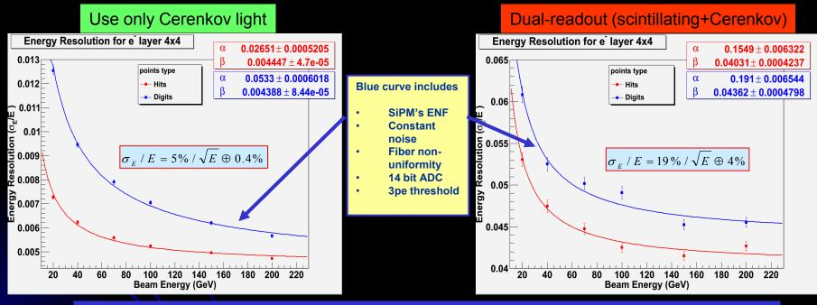
Using Cerenkov signal only for EM showers gives 5%/√E energy resolution while full fledged dual-readout gives only 19%/√E (including FEE effects)
