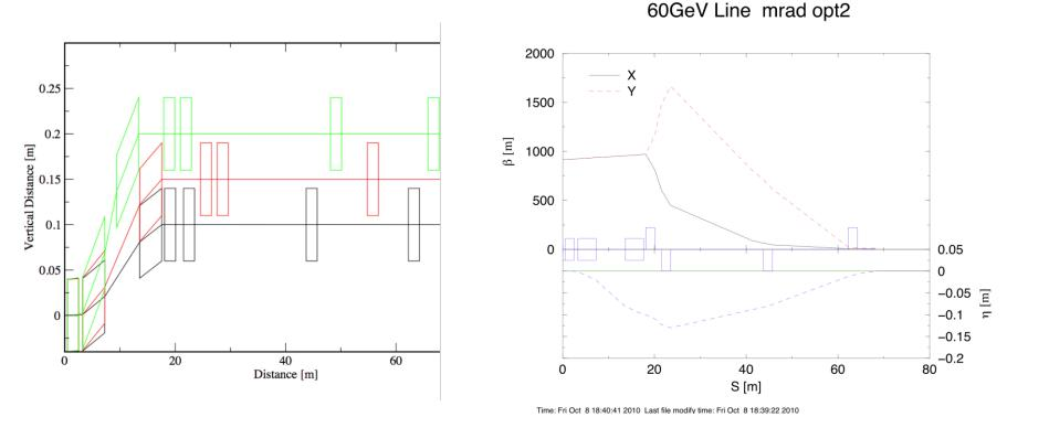
Optics functions of splitter for 20, 40 and 60 GeV beams and matching with the arc.
