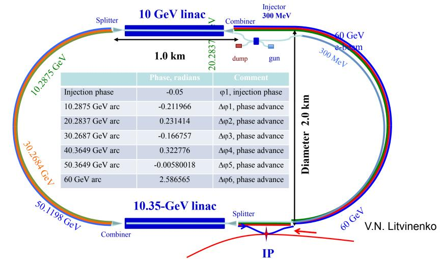
The electron bunch passes through the main linacs twelve times in the following sequence of phases: -0.05, -0.261966, -0.0305519, -0.197309, 0.125467, 0.119667, 3.08786, 2.85644, 3.0232, 2.70042, 2.70622, 2.87589. Finally, linac 1 will compensate for 0.922 GeV of the energy loss, while the linac 2 will compensate for the remaining 1.144 GeV.
