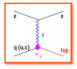
Or production of excited quarks, or of  $4^{th}$  generation quarks, via  $\gamma q Q$  (or Z q Q) couplings
