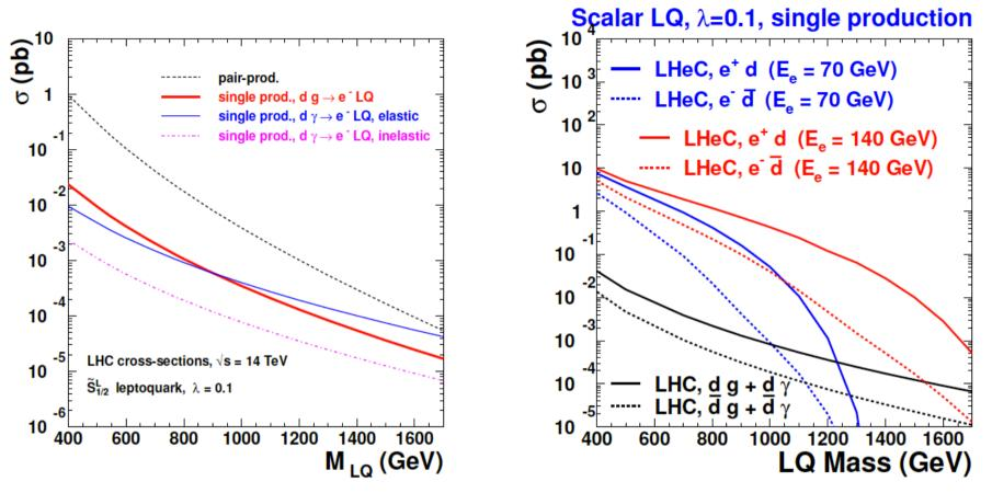
$\gamma q$  process increases the x-section for single LQ production at the LHC. But it is still much lower (O(100)) than the x-section in ep.
