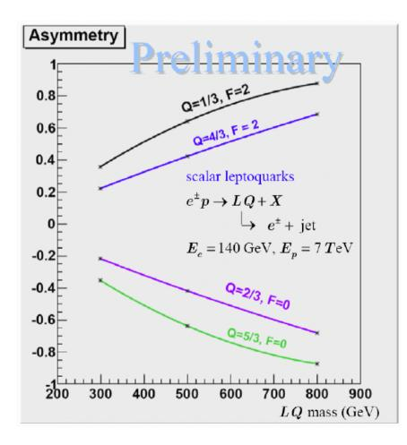
the charge asymmetry also allows to determine the electric charge of the LQ, i.e. the flavor of the quark to which the LQ couples.
