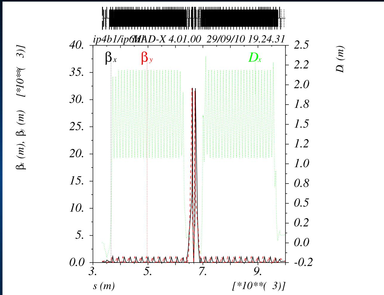
Made by Maxim based on Stephan's SLHC 3.0 ( $\beta_{x,y} = 0.1\text{m}$ ). Chromaticity corrected! Requires new triplets, D1, D2, Q4 and Q5.
