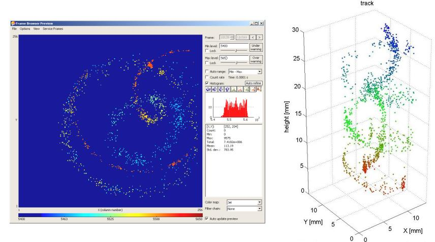
Projection of tracks of two β particles in B field (Pixelman software: IEAP, Prague)
