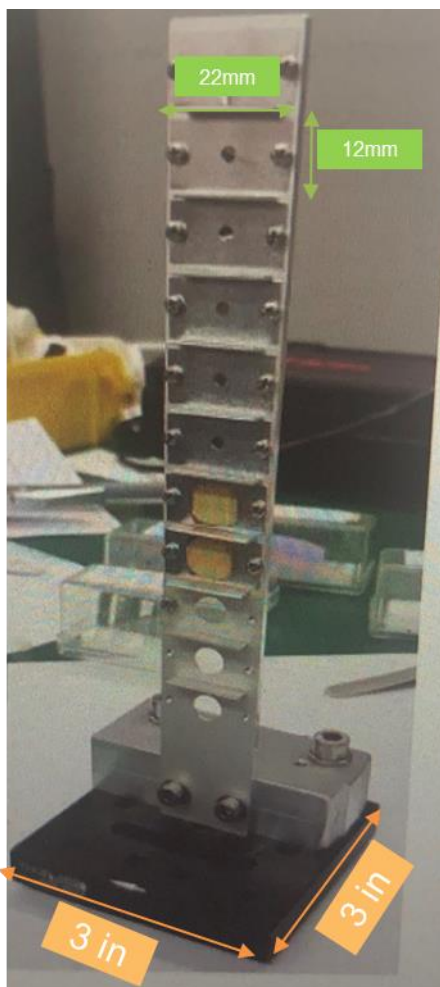
Figure 1: Sample holders installed on the kinematic mount.
