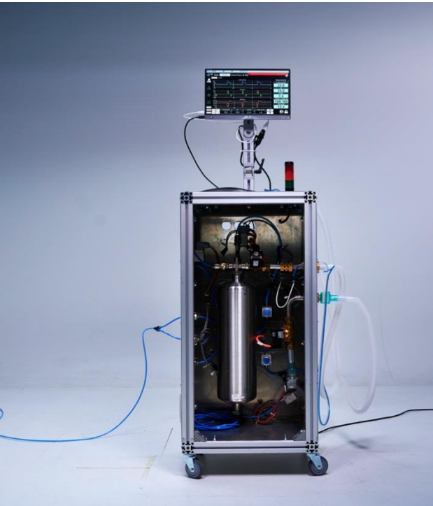
HEV (High-Energy Ventilator) design developed by members of the LHCb collaboration
