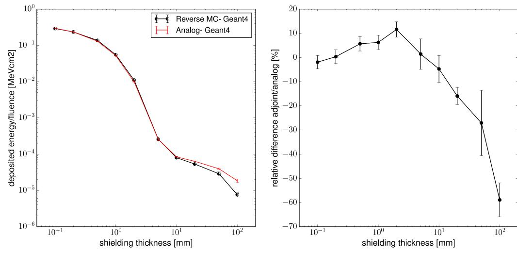
Discrepancy between Geant4 Reverse MC and Geant4 analog at thick shielding where the dose from secondary gamma dominates
