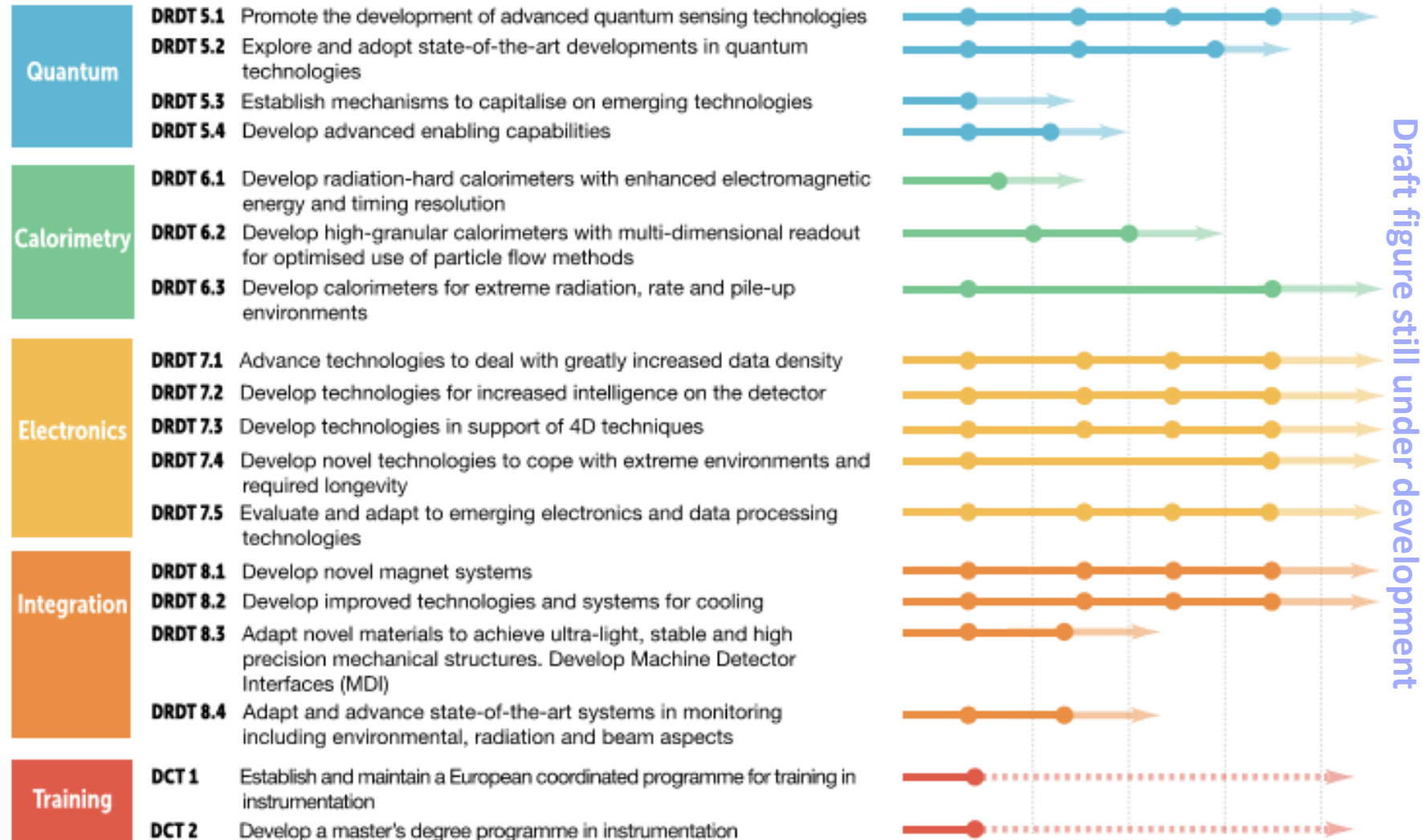
Figure 1: Detector R&D Themes (DRDT) and Detector Community Themes (DCT). Here, except in the DCT case, the final dot position represents the target date for completion of the R&D required by the latest known future facility/experiment for which an R&D programme would still be needed in that area. The time from that dot to the end of the arrow represents the further time to be anticipated for experiment-specific prototyping, procurement, construction, installation and commissioning. Earlier dots represent the time-frame of intermediate "stepping stone" projects where dates for the corresponding facilities/experiments are known. (Note that R&D for Liquid Detectors will be needed far into the future, however the DRDT lines for these end in the period 2030-35 because developments in that field are rapid and it is not possible today to reasonably estimate the dates for projects requiring longer-term R&D. Similarly, the dotted lines for the DCTs indicate that beyond the initial programmes, the activities will need to be sustained going forward in support of the instrumentation R&D activities).
