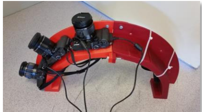
HD camera system for tunnel dome view
