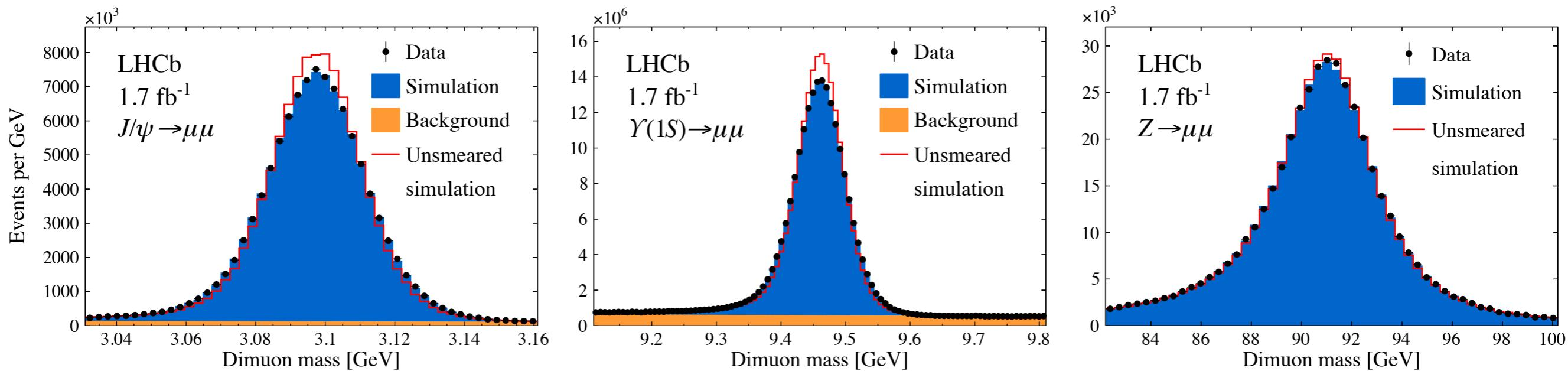
Simultaneous fit of  $Z$ ,  $\Upsilon(1S)$  and  $J/\Psi$  data (and simulation) in many categories<sup>1</sup>
