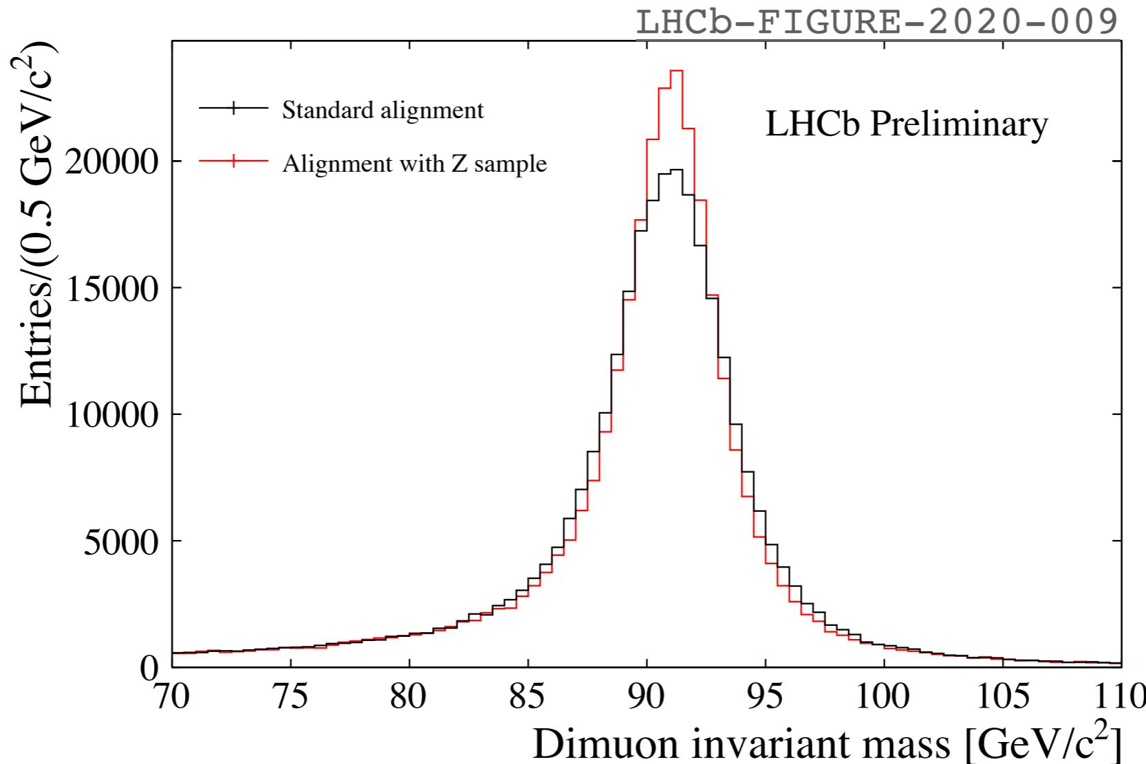
LHCb's successful real-time alignment and calibration was commissioned in Run-2 [JINST 14 \(2019\) P04013](#)
